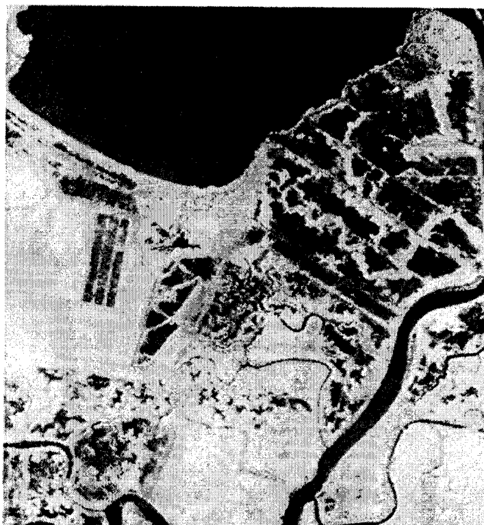
Figure 2. Band 68 (1.06 \mu m) after radiometric rectification.
