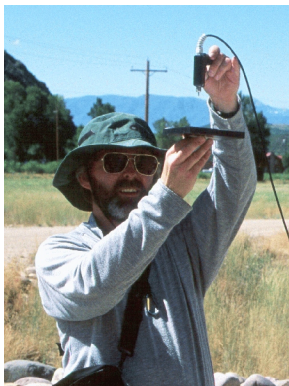
Figure 9d - Jordanelle Dam Calibration. Calibration of the reflectance target with the field spectrometer is important. Roger Clark holds the target high to minimize reflections from clothes, and makes his shadow side face the target. Roger's green Gortex hat has distinctive and sharp absorption bands. If any light from the hat contributed to the signal, inverse Gortex features would be seen in the spectra of the dam face, but no such features are seen in the data. Such checks are important to verify the accuracy of the calibration.
