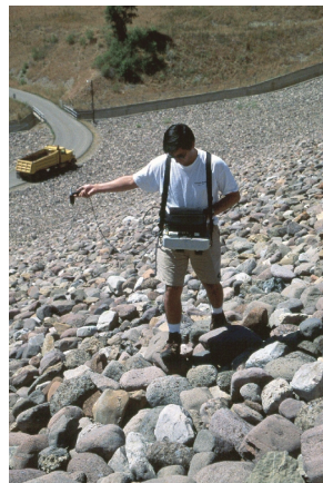
Figure 9b - Deer Creek Dam Calibration A. Ray Kokaly operates the field spectrometer on the Deer Creek dam face. Obviously, such a measurement is tricky because walking on large boulders is difficult.
