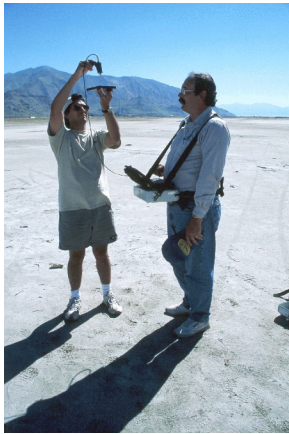
Figure 9a - Salt Flat Calibration. Spectralon calibration.
