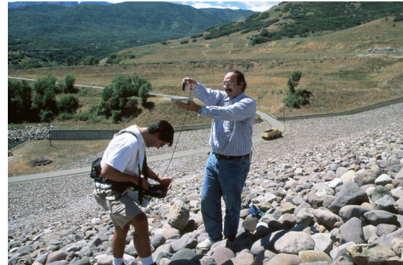
Figure 9c - Deer Creek Dam Calibration B. Frequent calibration of the field spectrometer is important. The constantly changing atmosphere and heat load on the instrument from sun and shadow as one moves around making measurements cause continual drifts. Here, Ray Kokaly operates the field spectrometer while Eric Livo holds the Spectralon reflectance standard. Eric holds the standard high and away from his body to reduce secondary reflections, and tries to position the standard so the shadow side of his body is seen by the standard.
