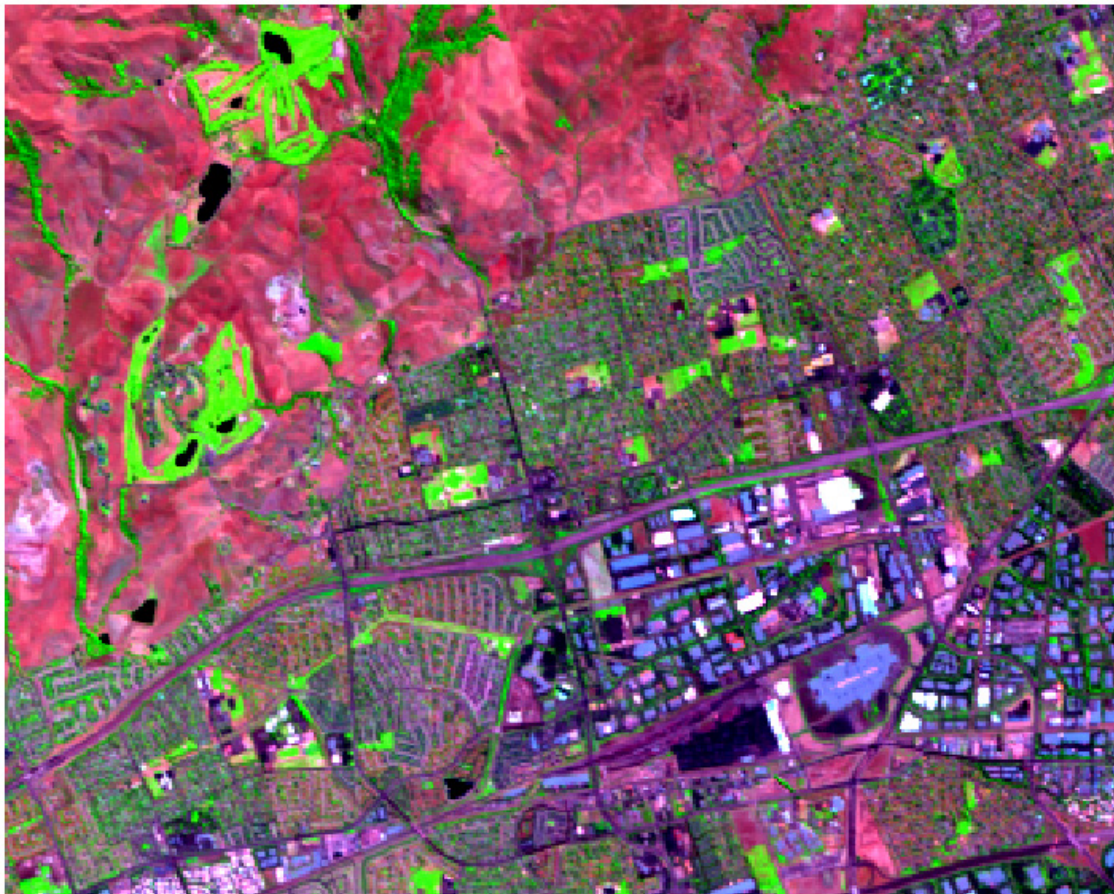
Figure 1. AVIRIS false color composite of Milpitas California acquired in 1997. The Red, Green and Blue layers correspond to the 2.21 \mu\text{m} , 0.81 \mu\text{m} and 0.66 \mu\text{m} wavelength bands respectively. The image is 6 x 8 km and each pixel is approximately 20x20 m. The spectral dimensionality of the mosaic of urban, suburban and undeveloped areas varies at scales larger and smaller than the Ground Instantaneous Field Of View (GIFOV) of the AVIRIS sensor.
